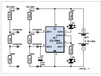
monitoring the LiPo propulsion batteries of radio control models that are used primarily in short range operation, such as indoor model helicopters.
