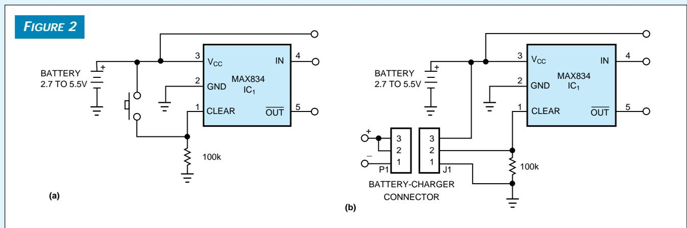
Other schemes for clearing  $IC_1$ 's output include an spst momentary pushbutton switch (a) and a connection through the battery-charger connector (b).
