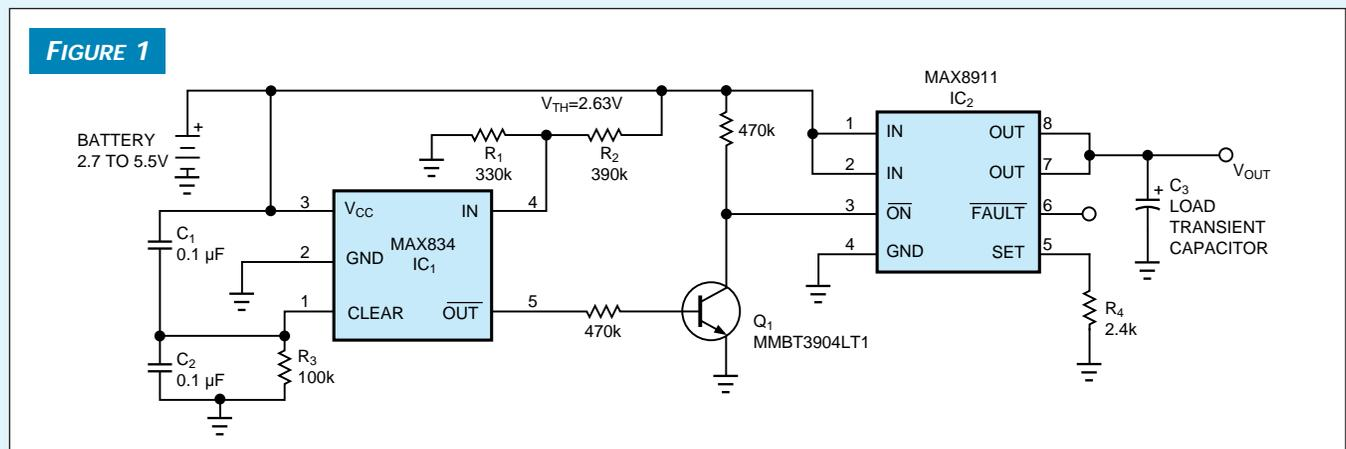
When the voltage reaches a minimum threshold established by  $R_1$  and  $R_2$ , the high-side switch,  $IC_2$ , turns off and disconnects the battery from the load.
