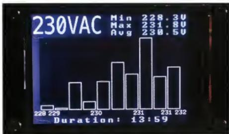
Fig.13: histogram plot of mains voltage. This gives you a good idea of which voltages the mains sits at most of the time relative to outliers. Note that the X-axis labels are rounded to the nearest volt while the data has sub-volt resolution.
