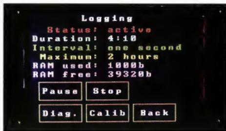
Fig.8: the logging status screen has also been improved since the first article. The same information is shown but there are now buttons to access the diagnostics screen and to perform automatic calibration. The button to dump logged data is not visible because you need to pause logging first.
