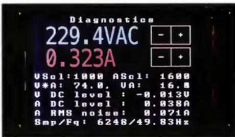
Fig.9: the diagnostic screen which shows the voltage and current readings with extra decimal places and allows fine adjustment of the scaling factors for both. It also displays the automatically calibrated calibration constants below, plus the sampling rate, measured frequency and pre-processing VA figures.
