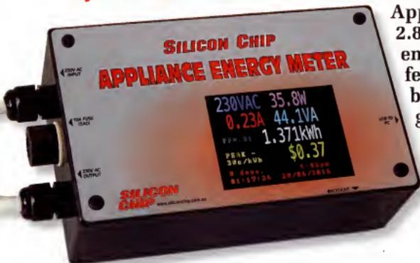
Last month we introduced our new Appliance Energy Meter. It uses a 2.8-inch touchscreen to display energy usage data and has handy features such as cost calculation based on time-of-day tariffs, graphing and logging. This second instalment will take you through the process of building the PCBs and assembling the whole unit, as well as describe some of the interesting features of the software.
