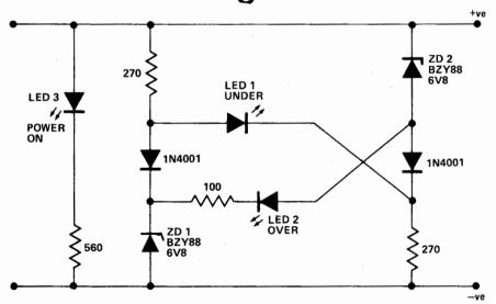
the input voltage increases to the extent that at the junction of ZD2, it exceeds the zener voltage of ZD1, plus the LED voltage of 1.6V, then
