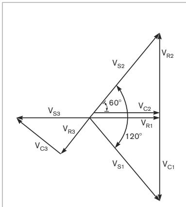
**Figure 2** When the voltages across  $R_1$  and  $C_2$  are equal,  $V_{C1} = -V_{R2}$ ,  $V_{C1} + V_{R1} = V_{S1}$ , and  $V_{C2} + V_{R2} = V_{S2}$ .
