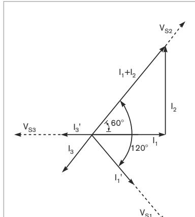
**Figure 4**  $I_3$  has half the magnitude and an exactly opposite direction to  $(I_1 + I_2)$  in **Figure 3**.
