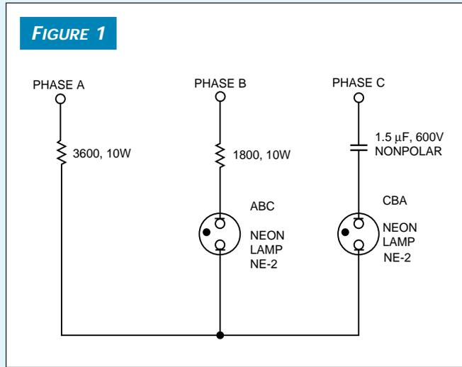
The brighter of the two neon lamps indicates the phase sequence, either ABC or CBA.
