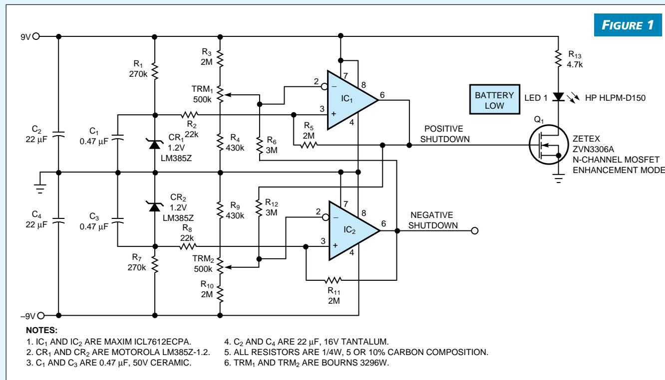
If either battery voltage in a two-battery supply drops below a preset limit, a Battery Low LED turns on.
