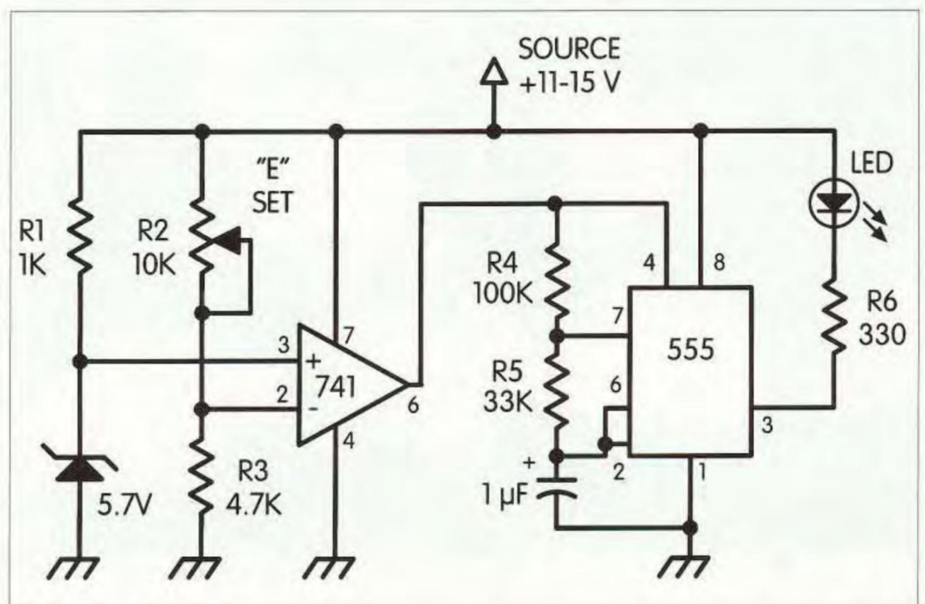
Fig. 1. Low battery voltage detector.
