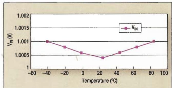
**Fig. 2.** The input voltage to the multiplier ( $V_{IN}$ ) in Fig. 1 varies as a function of temperature, reflecting the voltage reference's variation over temperature ( $V_{CC} = 5 \text{ V}$  and  $V_{SENSE} = 100 \text{ mV}$ ).
