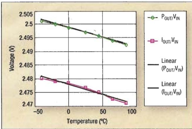
Fig. 3. The measured  $P_{OUT}/V_{IN}$  ratio in Fig. 1. is the same as the expected (linear) value of this ratio over temperature, unlike the measured  $I_{OUT}/V_{IN}$  ratio ( $V_{SENSE} = 100$  mV).
