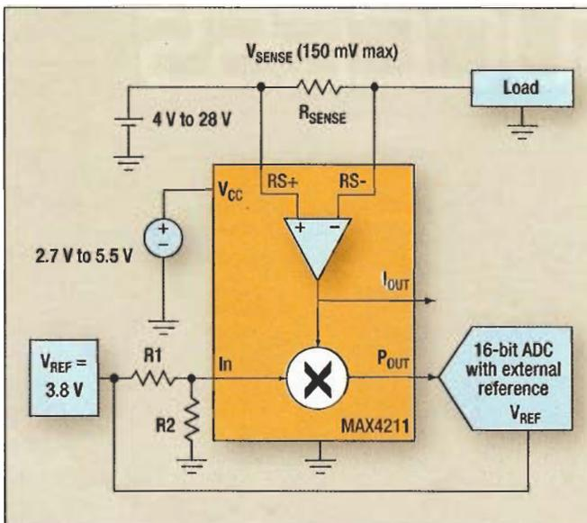
**Fig. 1.** This circuit uses a high-side power/current monitor (MAX4211) plus an ADC with external reference voltage to measure battery-charge currents with a high level of precision.
