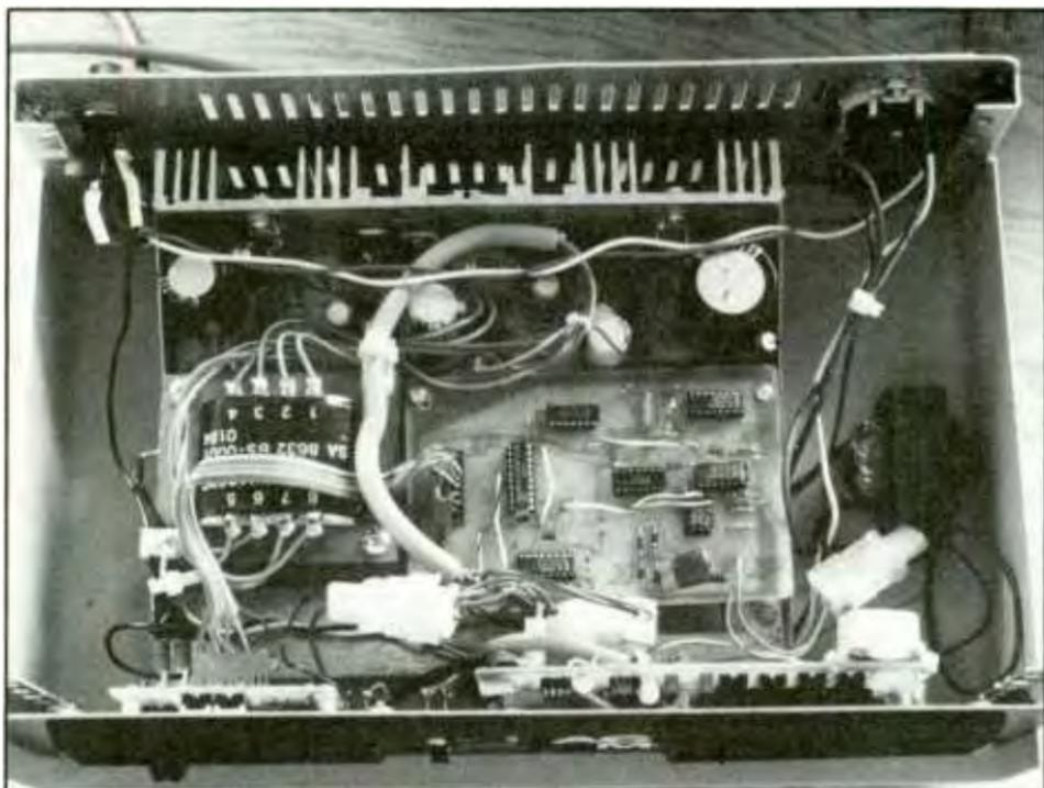
*Interior view of finished prototype of AC Line Monitor.*
