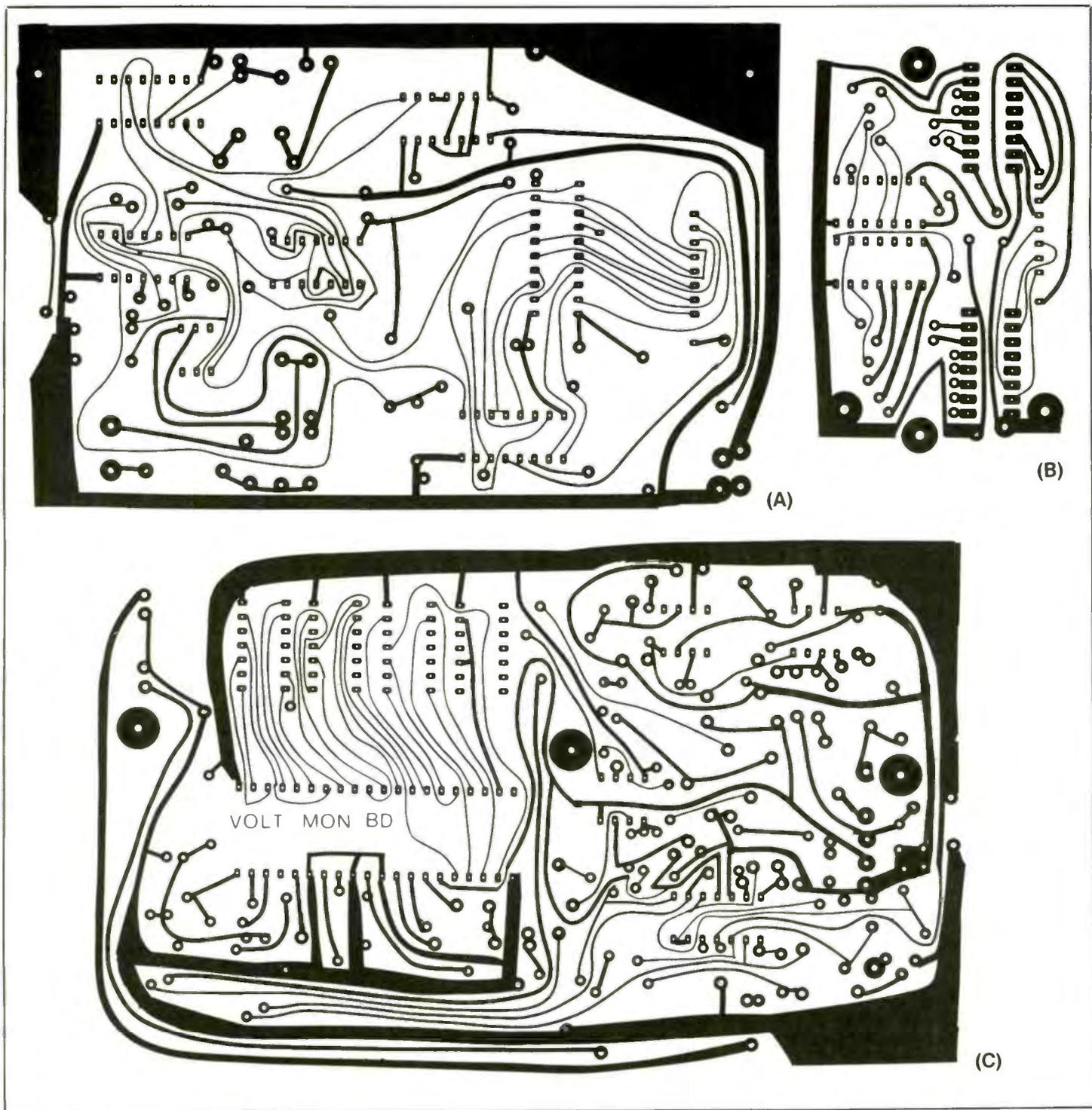
Fig. 5. Actual-size etching-and-drilling guides for printed-circuit boards: (A) frequency-counting module, (B) display module for frequency counter and (C) voltage-measuring module.
