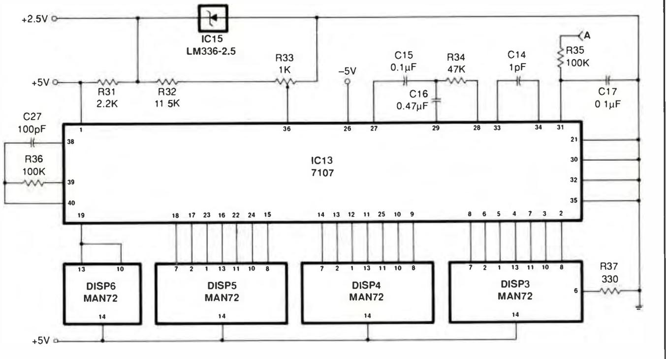
Fig. 4. Schematic diagram of voltage-measuring section, including four-decade numeric-display portion.
