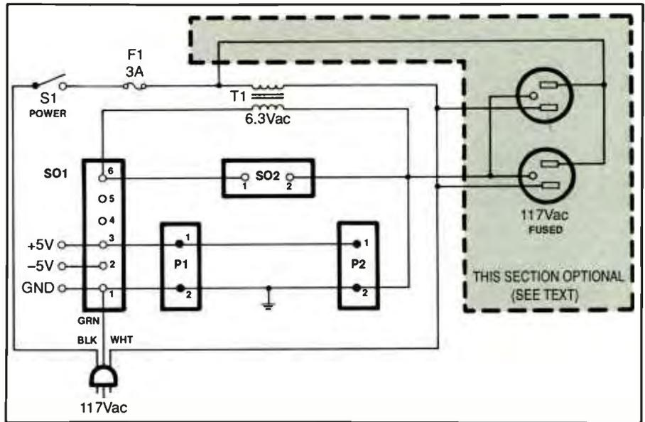
Fig. 1. Wiring diagram for power transformer and ac signal/dc power distribution to rest of project. Power supply can be built from scratch, or a ready-to-use power-supply module can be wired into circuit as shown. Ac receptacles shown at right are optional.
