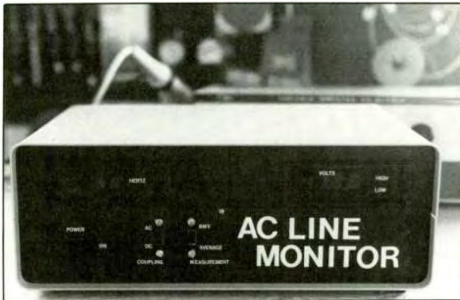
below preset levels. The LEDs light and buzzer sounds when the Monitor detects brief voltage sags and drops that would normally go unnoticed.
