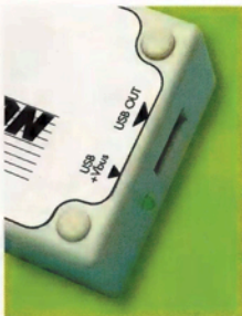
The power indicator LED protrudes through a hole in the end of the case, adjacent to the USB output socket (CON2).
