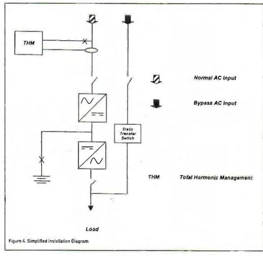
With its lower component count and higher MTBF, 6-pulse rectifiers offer end-users far greater efficiency and effectiveness. In relation to THM, combining 6-pulse rectifying technology with active harmonic conditioning produces reduced THDI levels and equally important, yet more difficult to quantify, enhancements in the end users' peace of mind.
