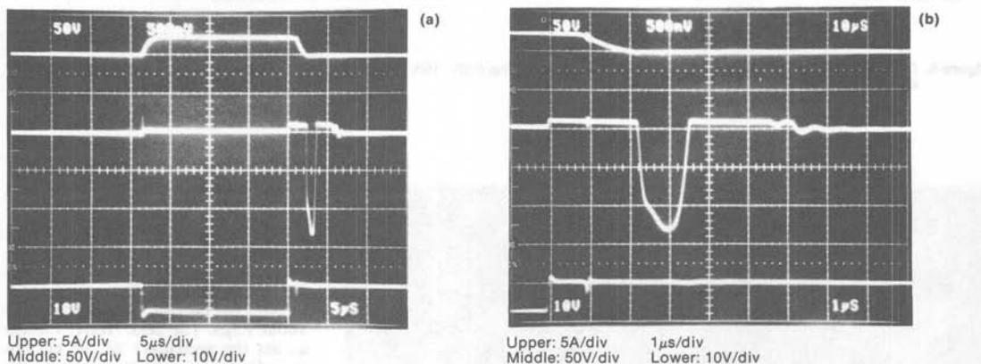
Figure 8. Base drive circuit waveforms for BIMOS switch of Figure 5 when switching 10A (a) 5 $\mu$ s/div (b) expanded to 1 $\mu$ s/div to show details of turn-OFF
