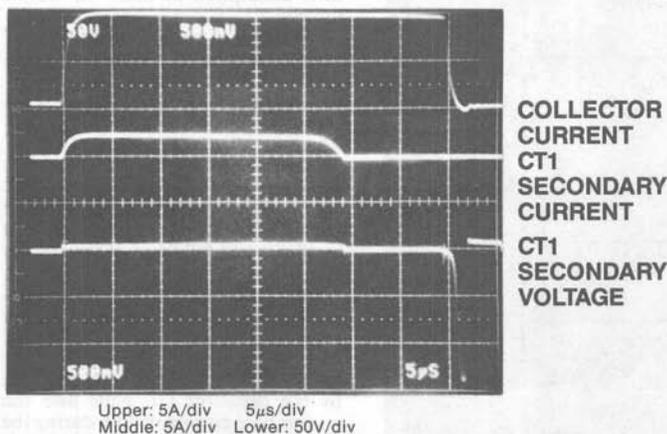
Figure 9. Base drive circuit waveforms for BIMOS switch of Figure 5 with conduction time greater than the 25 $\mu$ s maximum limit permitted by CT1
