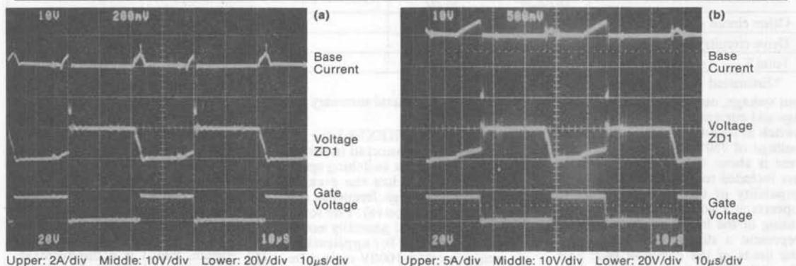
**Figure 23.** Base current, zener voltage, and gate voltage waveforms for BIMOS switch. 650V DC input.
