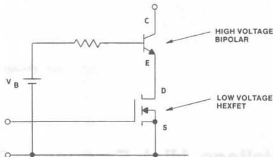
**Figure 2.** Cascode connection of HEXFET and bipolar
