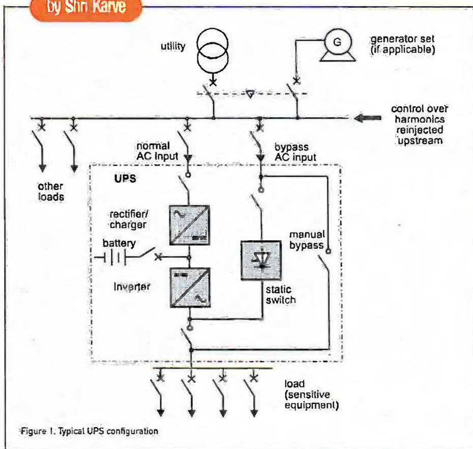
Figure 1. Typical UPS configuration
