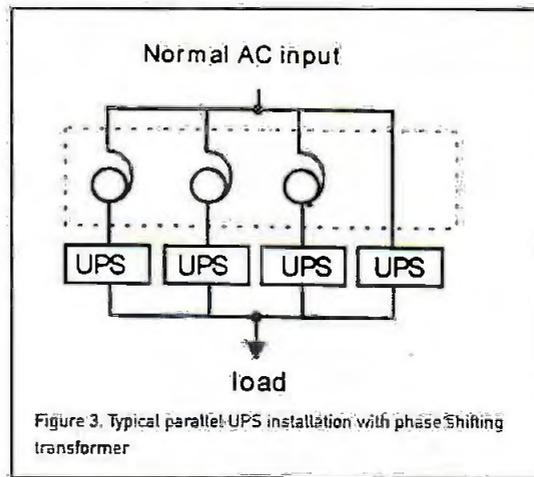
Figure 3. Typical parallel-UPS installation with phase shifting transformer
