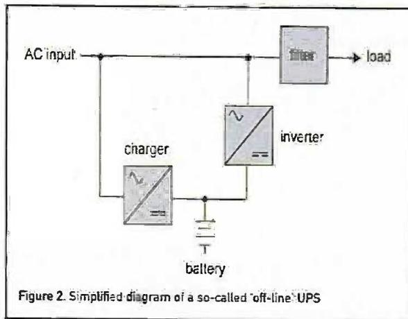
Figure 2. Simplified diagram of a so-called 'off-line' UPS
