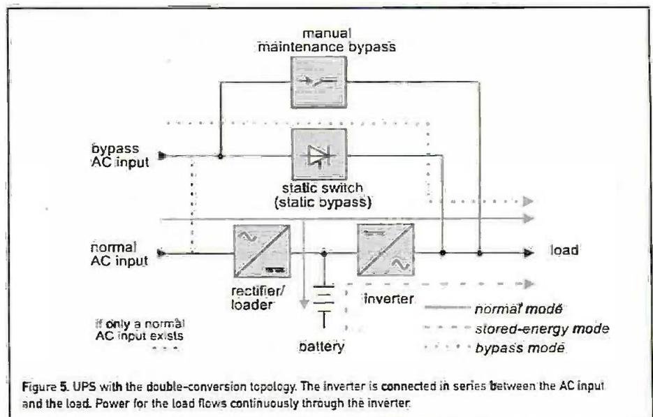
Figure 5. UPS with the double-conversion topology. The inverter is connected in series between the AC input and the load. Power for the load flows continuously through the inverter.
