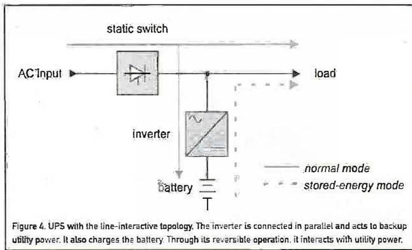
Figure 4. UPS with the line-interactive topology. The inverter is connected in parallel and acts to backup utility power. It also charges the battery. Through its reversible operation, it interacts with utility power.
