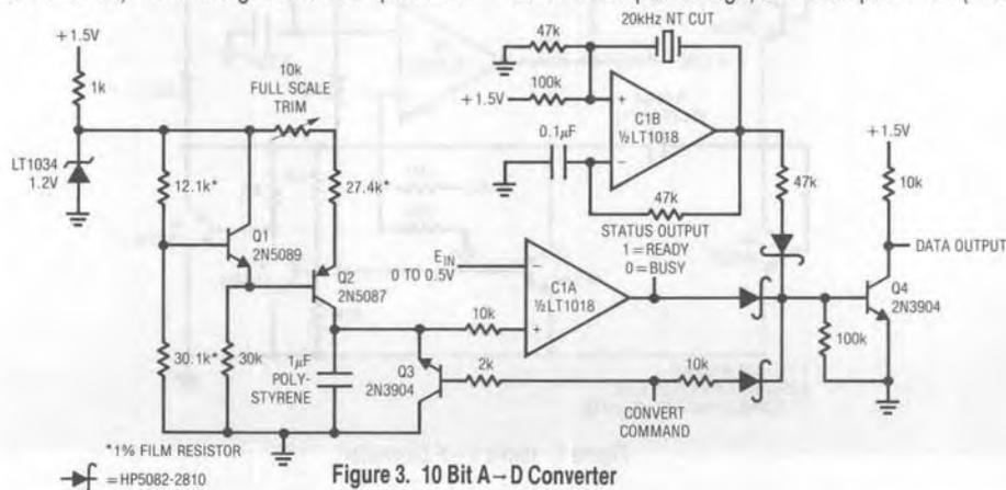
Figure 3. 10 Bit A-D Converter
