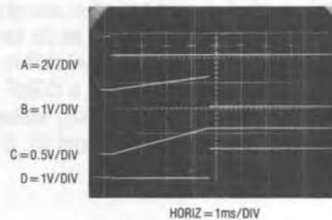
Figure 5. Sample-Hold Waveforms
