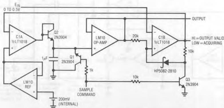
Figure 6. Sample-Hold Circuit
