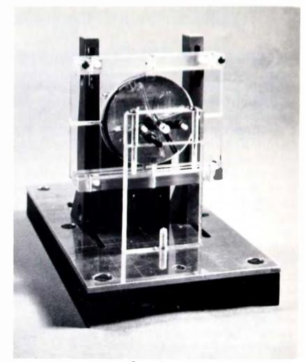
Photo Courtesy West Virginia University The World's first motor powered by energy from the Earth's electric field is shown above. It was developed by Dr. Oleg Jefimenko, professor of physics at West Virginia University. When the motor is running, the entire electret is shielded by a circular disk, which is one of the two mica-supported aluminum electrodes that rotate.
