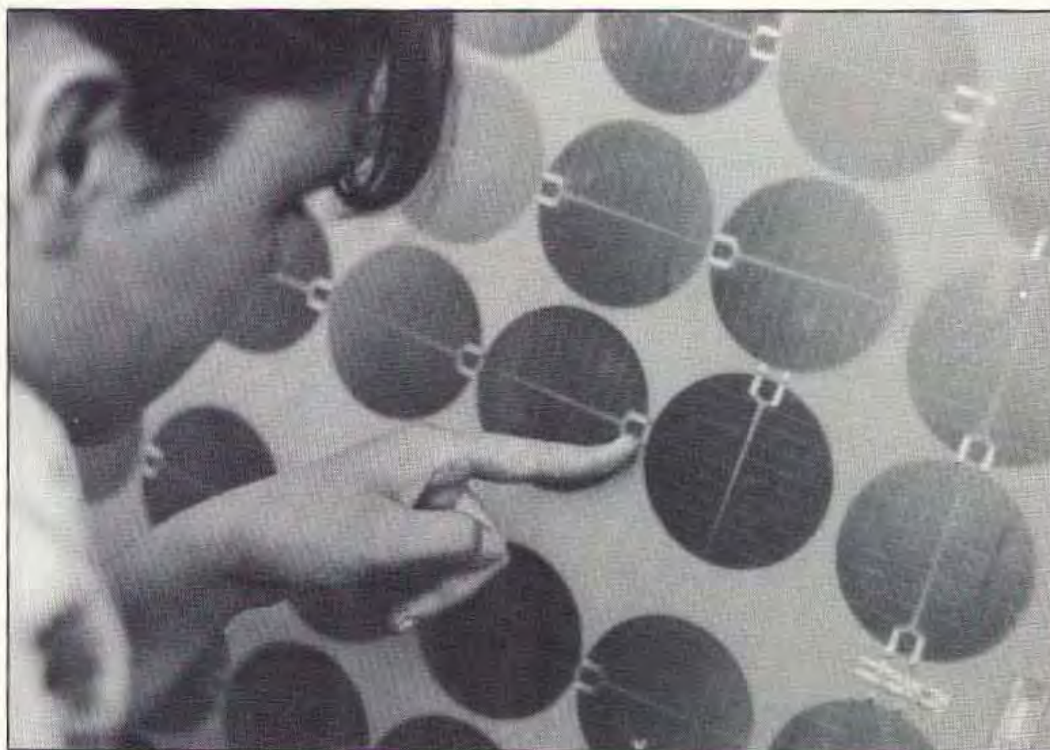
Photo A. Close visual inspection is the first step in testing surplus panels.
