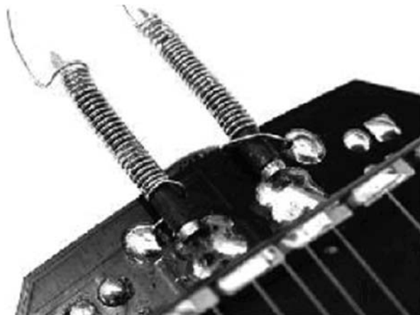
Finished sensor spring installation
