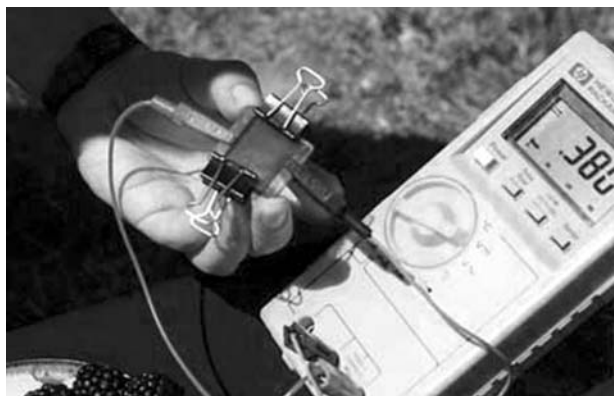
Figure 11-11 A closeup of the photochemical cell in action. Image courtesy Greg P. Smestad.
