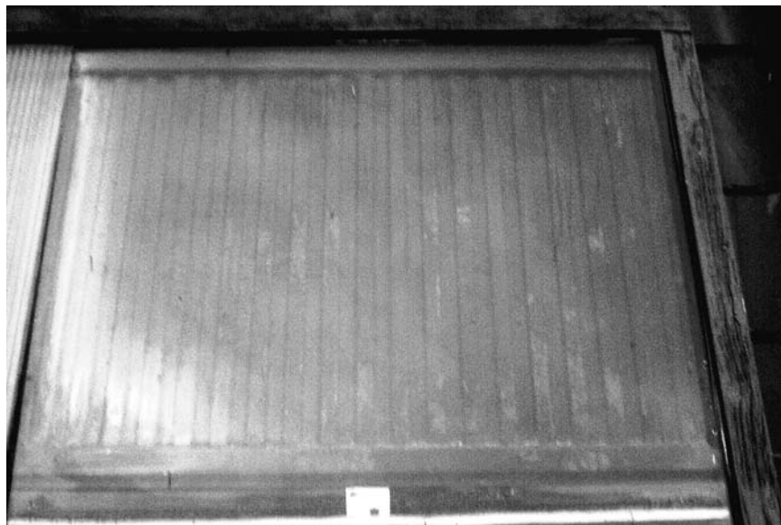
Figure 4-9 A recycled radiator collector.
