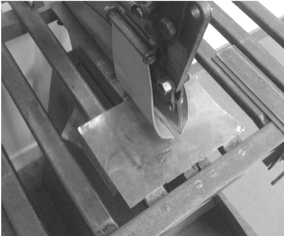
Figure 10-12 Cutting the copper with a guillotine.
