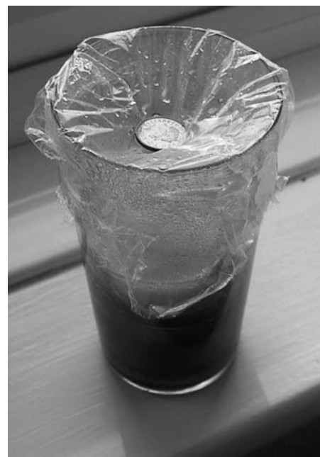
Figure 7-2 Demonstration solar still.
