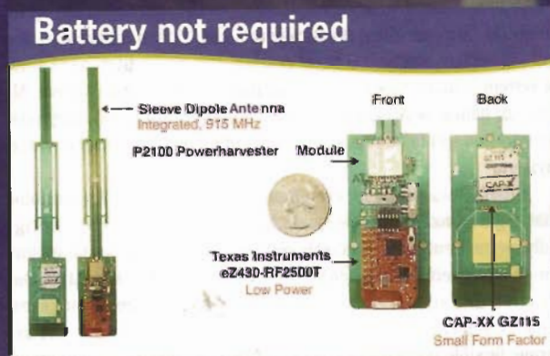
Here is an up-close look at a demonstration harvesting system that includes Powercast's P2100 Powerharvester chip. Also visible on the circuit substrate is a small form-factor capacitor and a low-power wireless board (TI eZ430-RF2500T).
