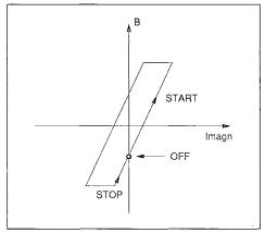
The timer is very precisely tuned in order to obtain precisely 10ms delay between two gate pulses. As a result, the triac is driven symetrically in both phases so continuous voltage in the transformer is avoided.
