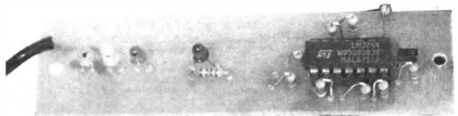
Layout of components on the completed circuit board. The method of mounting the p.c.b. on the removable panel and positioning of the fuseholder is shown below.
