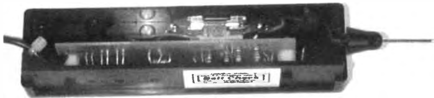
Completed "checker" with the removable side panel, holding the p.c.b., slotted into position ready for closing-up the box.
