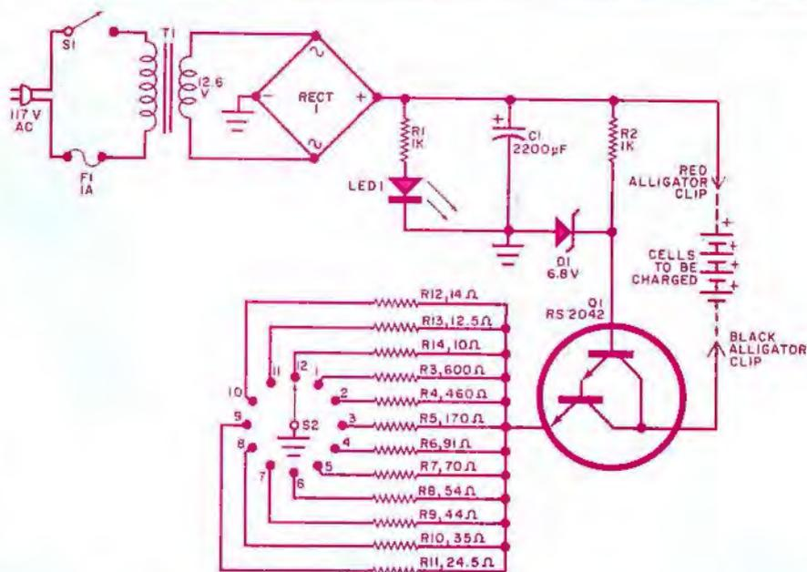
Fig. 1. Schematic shows how zener *D1*, Darlingtion *Q1*, and resistors *R3* through *R14* form constant-current source which regulates battery charging.
