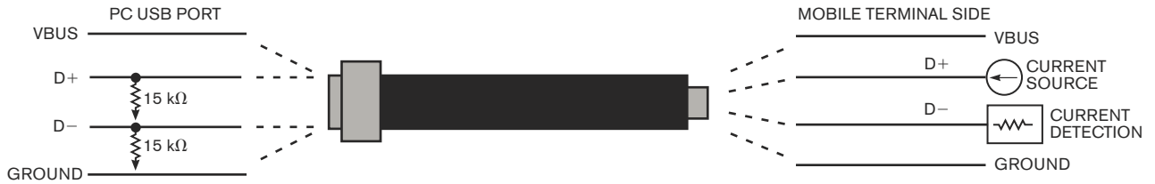
Figure 4 If you use a PC's USB port for battery charging, the D+ and D- pins do not short together as they do in the wall-mounted charger. In addition, a 15-k \Omega resistor connects each of the pins to ground.
