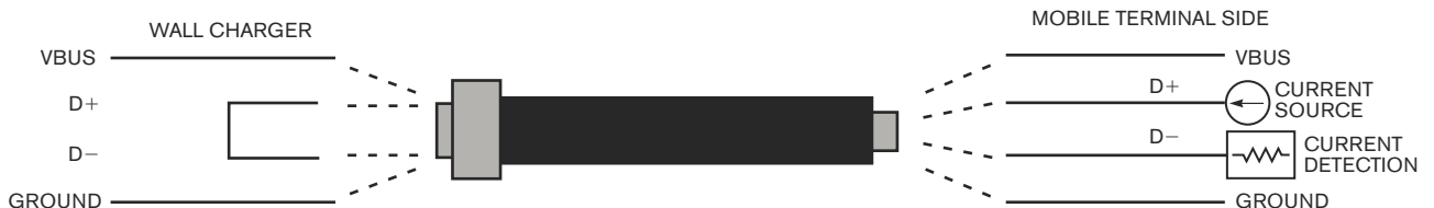
Figure 3 To control charging current, a new spec from the USB Implementers Forum calls for wall-mounted battery chargers to implement this design, which connects the USB connector's D+ and D- pins but does not otherwise connect them.
