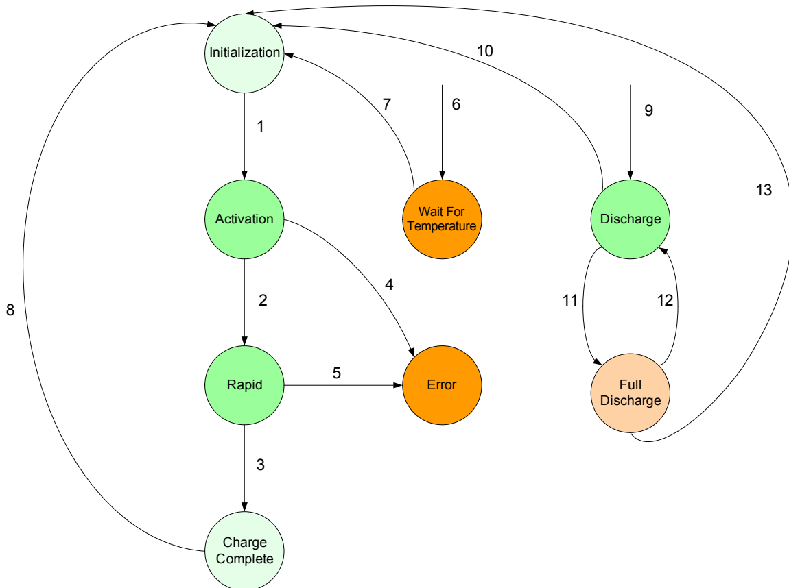
Figure 8. Two-Cell Battery Charger State Diagram
