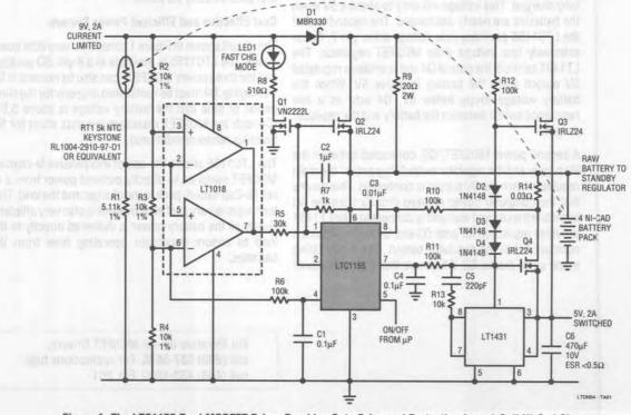
Figure 1. The LTC1155 Dual MOSFET Driver Provides Gate Drive and Protection for a 4-Cell Ni-Cad Charger and Regulator limited wall unit is switched directly into the battery pack through an extremely low resistance MOSFET switch, Q2. The gate drive output, Pin 2, generates about 13V of gate drive to fully enhance Q1 and Q2. The voltage drop across Q2 is only 0.17V at 2A and, therefore, can be surface mounted to save board space.
