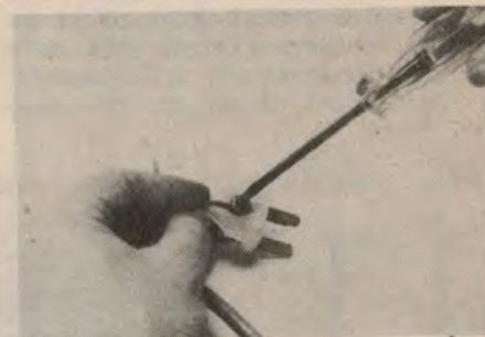
3. Tighten terminal screws firmly.
