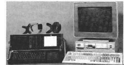
FIG. 7—THE DRANETZ SERIES 656 Disturbance Waveform Analyzer. Note the built-in CRT, full keyboard, dual floppies, and thermal printer.
