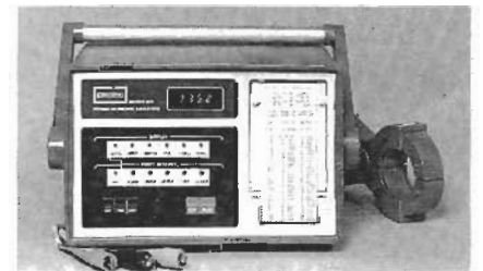
FIG. 5—THE DRANETZ SERIES 901 POWER HARMONIC ANALYZER, similar to a BMI 2400. In one printout for a instant in time, the device records line voltage, the current used, total power, power factor, harmonic power, fundamental power, and a breakdown of the power in the individual harmonic frequencies above the fundamental (in other words, its spectral content).
