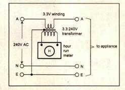
three and 12 volts, as this rating only affects the lowest power the hour meter will respond to. The current rating of this winding should equal or exceed the full load current being measured. A refrigerator draws around 300 watts or 1.2A at 240 volts, so the winding must be able to carry that current.
