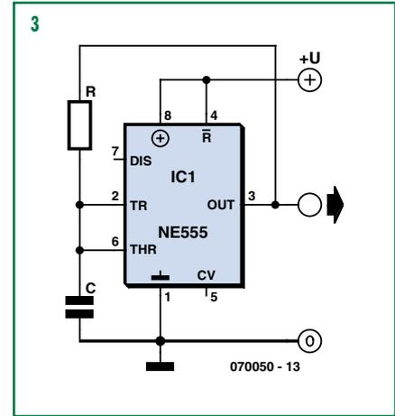
So there is an opportunity to do better still. And this is shown in **Figure 3**. This extremely simple schematic shows a clock generator using an NE555 with a 50% duty ratio in its minimal form. It requires only three com-
