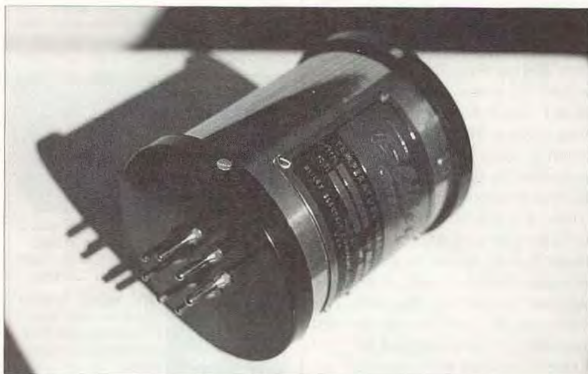
Photo B. Bliley crystal oven removed from SRT-14.
