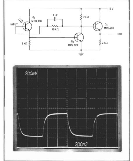
**Speedy.** Collector-to-base capacitance of phototransistor  $Q_1$  is reduced by employing epitaxial device (MRD 300) and high-gain negative feedback ( $Q_2$ ), so that operating speed can be increased. Emitter-follower  $Q_3$  provides low-impedance output. Photograph shows typical output response.
