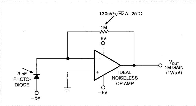
Figure 1 A conventional 1-M $\Omega$  transimpedance amplifier exhibits 130 nV/ $\sqrt{\text{Hz}}$  of output noise, even with a noiseless op amp. Cooling the resistor reduces the noise, but can you do better without cooling?
