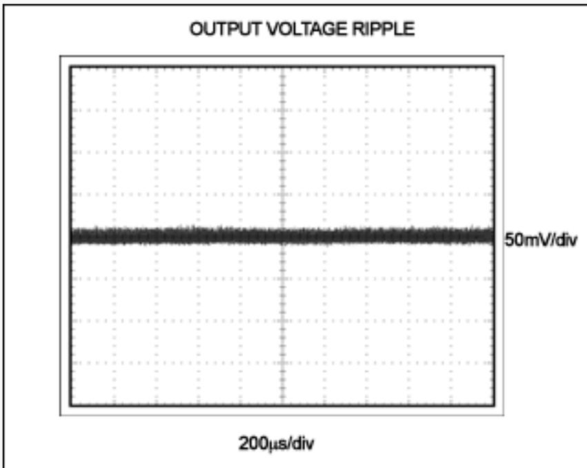
Figure 4. This graph demonstrates the output voltage ripple for Figure 1's circuit with  $V_{OUT} = 71V$ ,  $I_{OUT} = 1mA$ , and a  $10\mu F$  electrolytic capacitor in parallel with the  $1\mu F$  output capacitor. The vertical axis is  $50mV/div$  and the horizontal axis is  $200\mu s/div$ .
