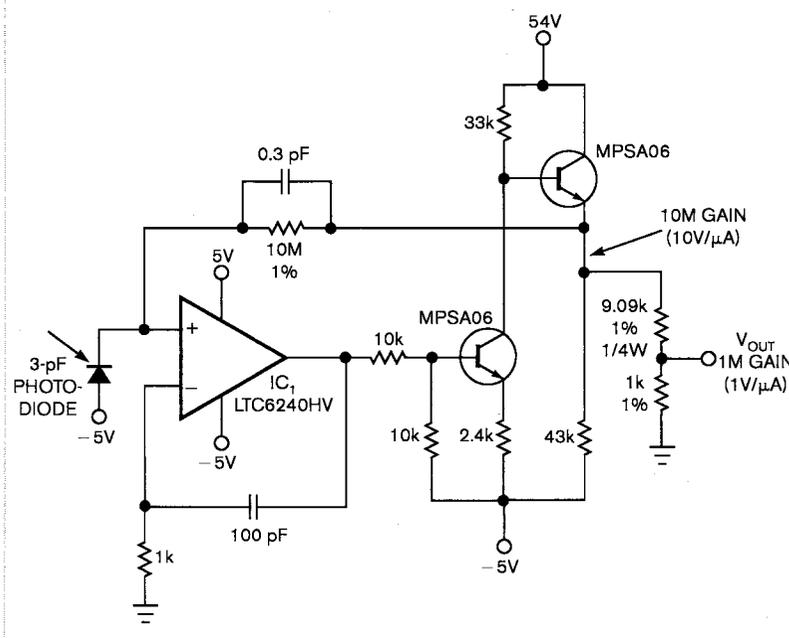
Figure 2 This effective 1-M $\Omega$  transimpedance amplifier has only 43 nV/ $\sqrt{\text{Hz}}$  of output noise. The circuit takes 10 times the high amplifier gain and then attenuates by a factor of 10. The LTC6240 has low current and voltage noise. The discrettes allow for high output swing at the 10-M $\Omega$  gain node, so that a 0 to 5V output swing remains after attenuation.
