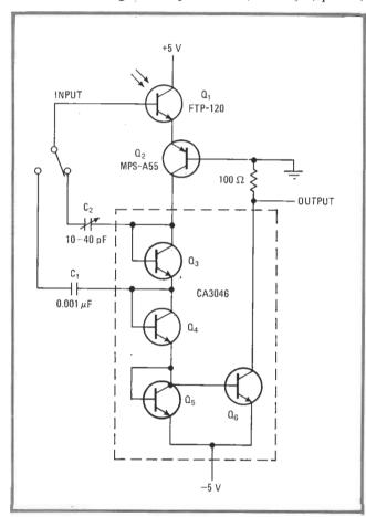
**Compensation.** Junction capacitance of  $Q_1$ , which is not sufficiently reduced despite cascode connection  $(Q_1, Q_2)$ , is greatly lowered by applying feedback to base. This allows a rapid discharge of  $Q_1$ 's base-to-emitter capacitance during signal conditions, which acts to increase the phototransistor's high-frequency response.
