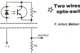
Two wires for opto-switch F. Arfort, Melton South, Vic.
