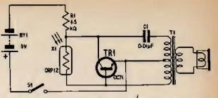
The detector unit is portable and the infra-red sensor is housed in a pen and covered by an infra-red filter such as Everine black tile. The sensor is then attached to the detector unit by microphohe cable. J. Walker, Dunfermline, Fife.
