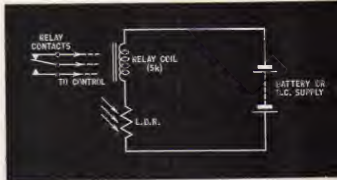
Fig. 4. A photoconductive cell (light-dependent resistor) can be arranged in this simple circuit to provide an effective light-operated switching action
