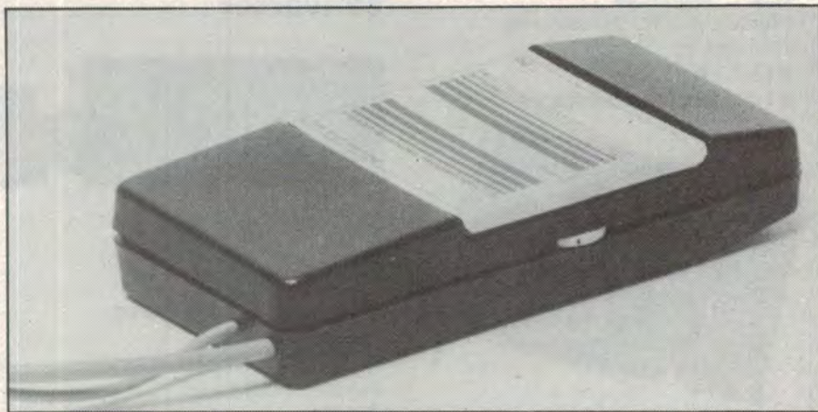
The transmitter unit, housed in the same compact plastic case as the receiver.
