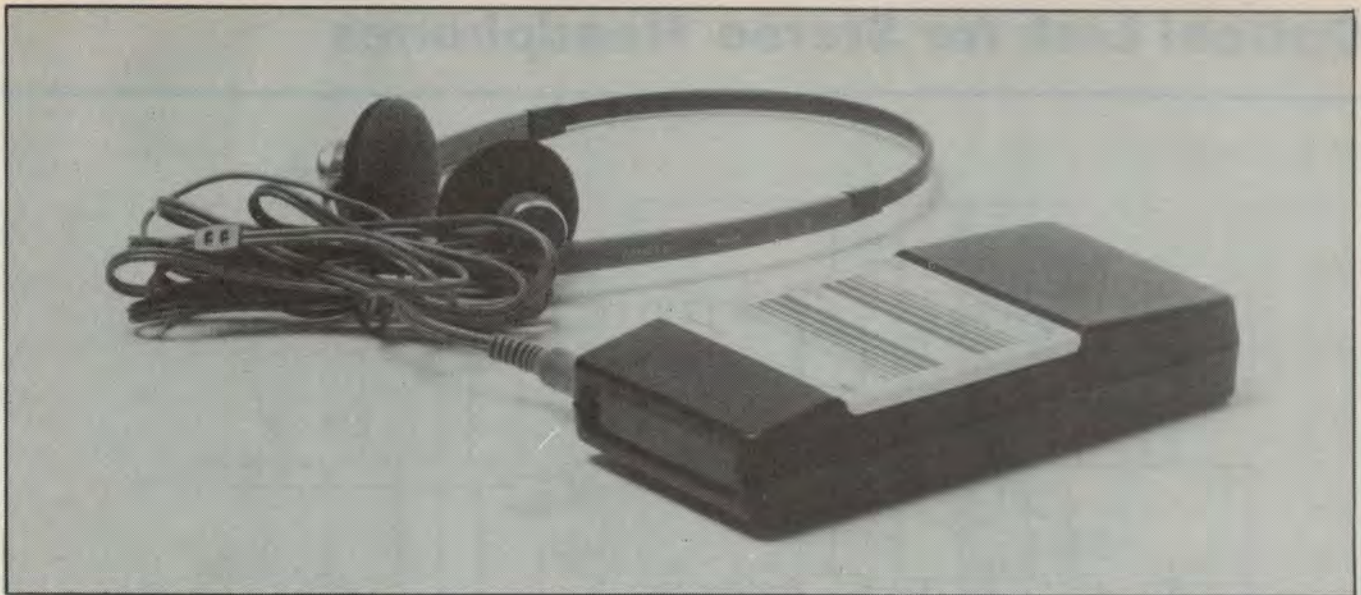
The receiver unit, with typical lightweight headphones. It runs from a standard 9V battery.
