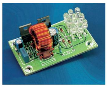
this converter supplies a constant current instead of a constant voltage. A resistor in series with the LEDs produces a voltage drop that depends on the current through the LEDs. This voltage is compared inside the IC to a 1.25-V reference value, and the current is held constant at 18.4 mA (1.25 V  $\div$  68  $\Omega$ ).
