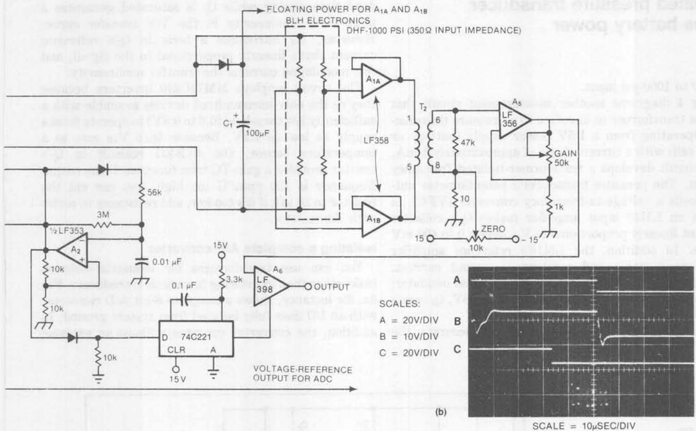
**Fig 3**—In addition to supplying floating drive to the strain-gauge bridge, this network furnishes transducer output-signal amplification (a). Because the Sample command—trace C in (b)—occurs while T<sub>2</sub>'s output is settled, network output is a dc representation of pressure-transducer output.
