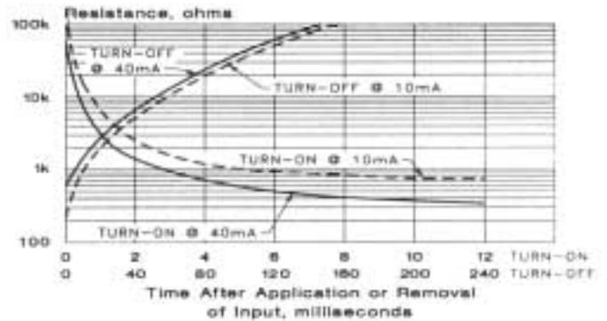
Output Resistance vs. Input Current
