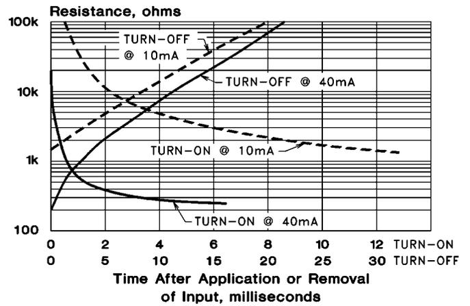
Output Resistance vs. Input Current
