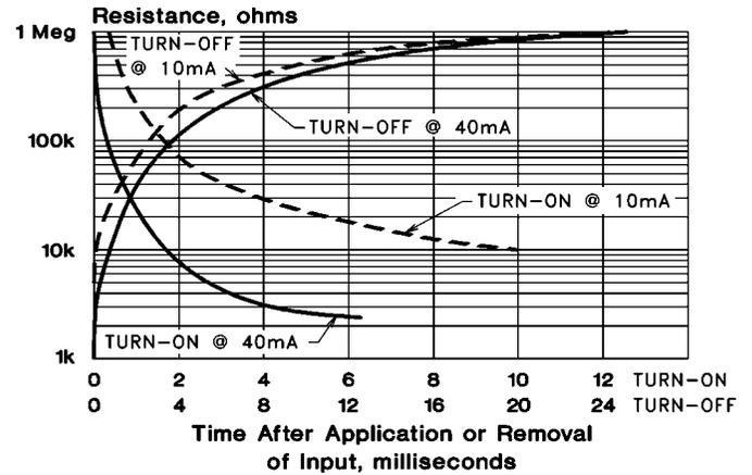
Output Resistance vs. Input Current
