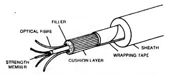
Fig. 3: Long wavelength, four-core layer type optical fibre cable structure.
