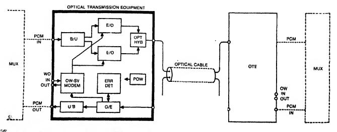
Fig. 4: Configuration of an optical digital transmission system.
