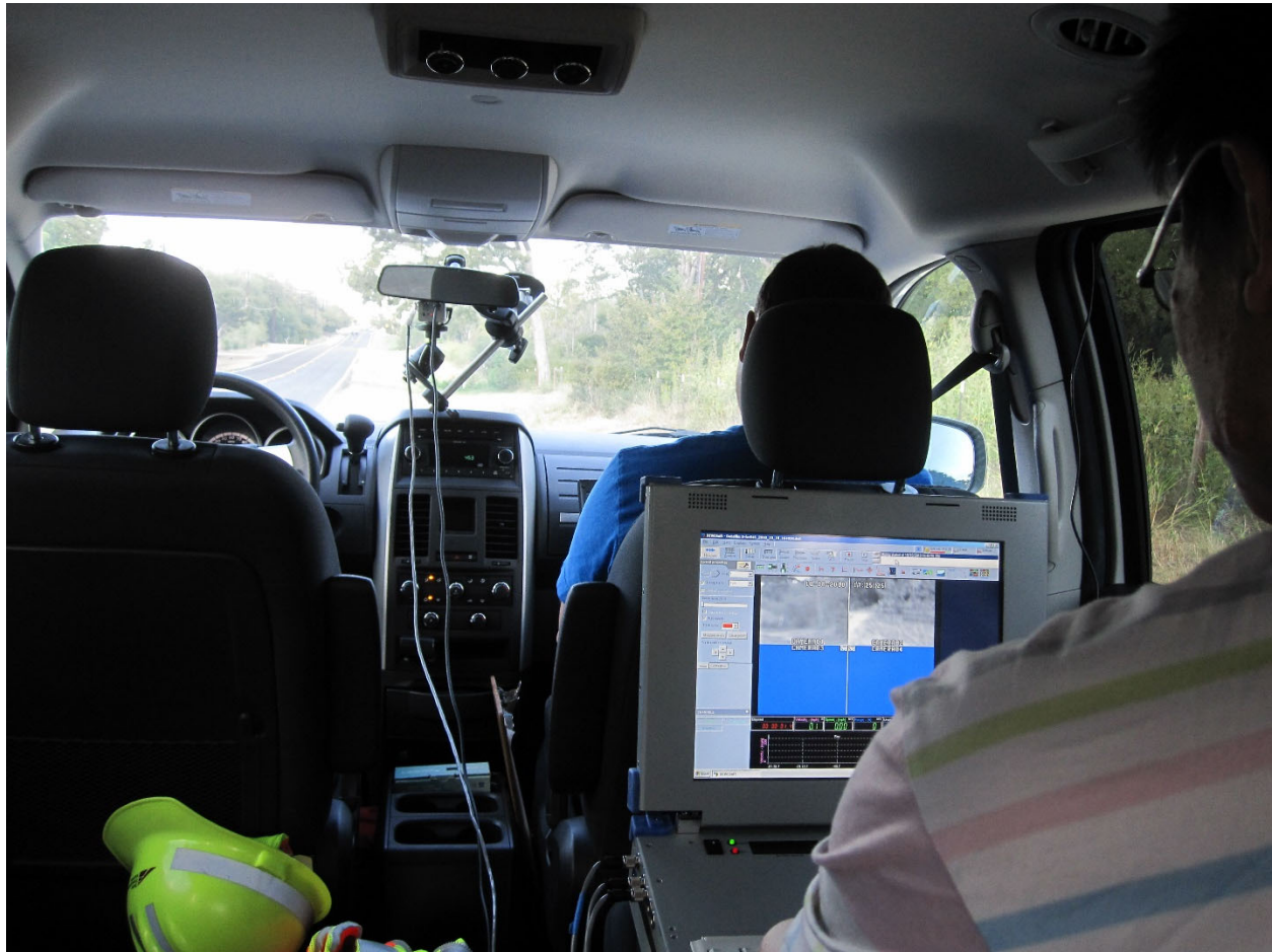
FIGURE 2 Cameras, sensors, and data acquisition unit in an instrumented vehicle. (Image Credit: Marcus Brewer)
