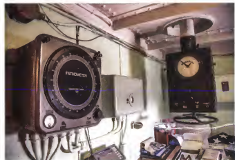
Fig.9: the Dorsey Fathometer as installed on the SS John W. Brown, a US Liberty Ship during World War II.
