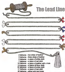
Fig.2: a lead line or sounding line showing different markers at traditional depths of 2, 3, 5, 7, 10, 13, 15, 17 and 20 fathoms. A fathom is today defined as exactly six feet or 1.8288m. Fathoms and feet are still used on US nautical charts whereas other countries use metres.
