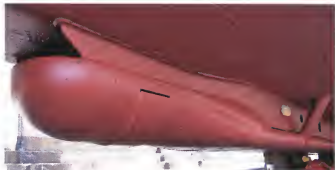
Fig.19: a Kongsberg multibeam echo sounder mounted on survey vessel. Note the partially visible person at bottom right for an idea of its size.
