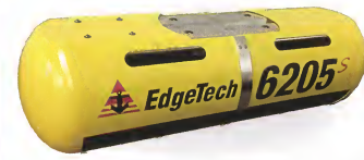
Fig.23: the 208 x 244 x 759mm EdgeTech 6205S hybrid multibeam and side scan sonar instrument. It operates at 230, 550, 850 and 1600kHz and has a range of 250m at the lowest frequency and 35m at the highest, used for side scan. For multibeam work at 230kHz, it has a swathe width of 400m.
