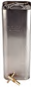
Oxygen generators – a sealed can containing sodium chlorate to produce oxygen by chemical decomposition.
