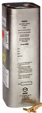
Oxygen generators – a sealed can containing sodium chlorate to produce oxygen by chemical decomposition.
