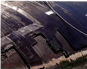
An example of tiles that have become detached from a nuclear submarine due to improper attachment. When attached correctly they are extremely difficult to remove.
