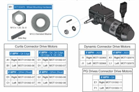
The Complete Drive Motor includes the Wheel Mounting Hardware (M1). They DO NOT include the Motor Mounting Hardware. The model specific hardware MUST be selected separately.
