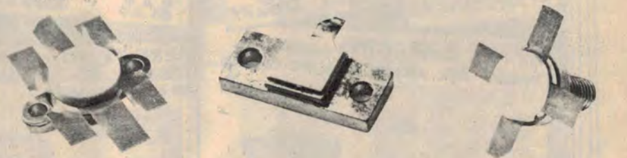
Some of the fairly common types of devices constructed using Beryllium oxide are shown above. RF power transistors use the material as a heat transfer material between the chip and the copper stud. Stripline terminations — such as the central device in the upper group and the central device in the lower row — are less common but have construction similar to the RF power transistors. These devices are perfectly safe to handle providing you do not do any of the things suggested in the pictures on the opposite page.
