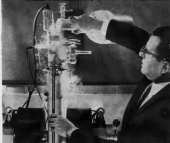
Bell Labs' engineer submerges specimen of a new ternary semiconductor with liquid nitrogen during a typical materials research experiment. Typical properties being measured are carrier mobility, resistivity and magneto-resistivity.
